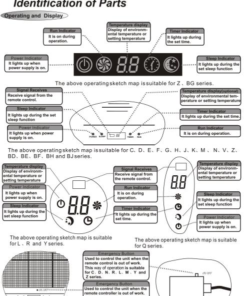
Remarks: When remote control is not working properly, open the panel and you can see emergency button there, (see above picture). The emergency button for 15K, 16K, 18K, 22K, 24K 28K and 30K series is at the top right, see "ON/OFF" button there.
